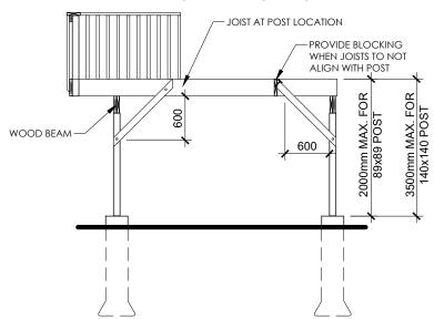
FREE STANDING DECKS GREATER THAN 600mm ABOVE GRADE SHALL RESIST LATERAL LOADING AND MOVEMENT. ALL POSTS MUST BE BRACED WHERE THE DECK WALKING SURFACE TO FINISHED GRADE EXCEEDS 1.5m (5').
