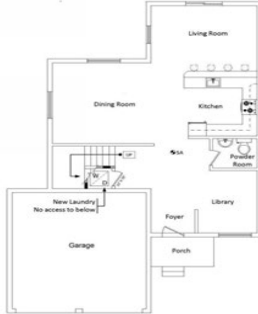
Figure 2 - Existing Main Floor Layout Modified
