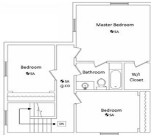
Figure 3 - Existing Second Floor Layout
