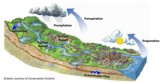
Figure 5: Components of a Water Balance
