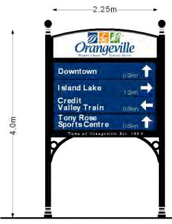
\*print ready digital graphics for all sign face aitwork required prior to manufacture - sign post sizing and proposed concrete footing to be reviewed and approved by a structural engineer licensed to practise in Ontario
