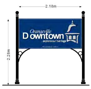
\*print ready digital graphics for all sign face artwork required prior to manufacture - sign post sizing and proposed concrete footing to be reviewed and approved by a structural engineer licensed to practise in Ontario
